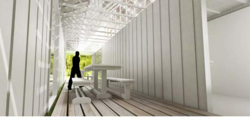
We propose a combination of re-usable structures (shipping containers), prefabricated components (e.g., the truss roof), and locally available materials, such as soil for the modular edible gardens. All components are designed to fit inside the two shipping containers, enabling the units to be moved with minimum effort or additional materials. Units can remain sited or be transported seasonally.
