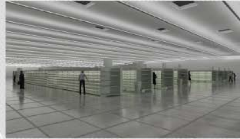
Ceiling Lighting at 25% Shelf Lighting at 0.25W/ft
